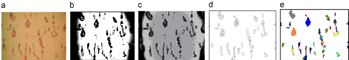
Fig. 6. Segmentation results of ferrograph image 2. (a) Original image, (b) K-means, (c) FCM, (d) marker-watershed, and (e) CWACA segmentation.
