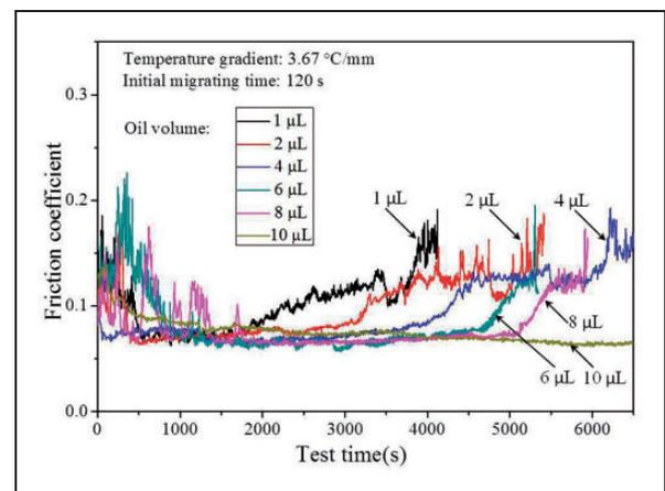
**Figure 8.** Evolution of friction curves under different oil volumes at temperature gradient of  $3.67^{\circ}\text{C}/\text{mm}$ .
