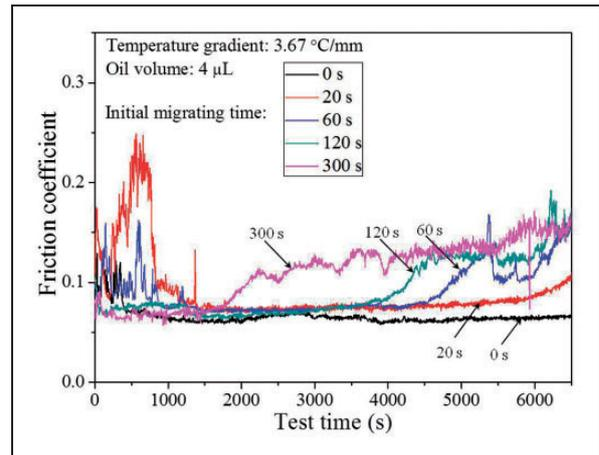
**Figure 10.** Evolution of friction curves under different initial migrating times at temperature gradient of  $3.67^{\circ}\text{C}/\text{mm}$ .
