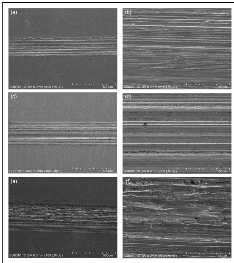
**Figure 11.** SEM images of the worn substrate surfaces with different initial migrating times. 20 s (a and b), 60 s (c and d) and 120 s (e and f).
