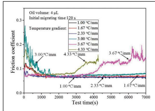
**Figure 5.** Evolution of friction curves under different temperature gradients.
