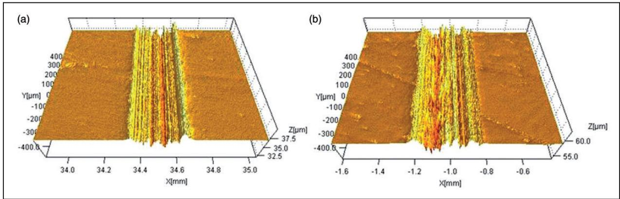
**Figure 12.** Three-dimensional (3D) morphologies of wear tracks with different initial migrating times. (a) 20 s and (b) 120 s.
