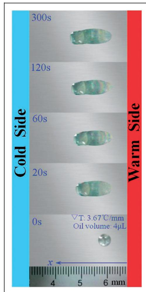
**Figure 2.** The image of oil migration behaviors recorded with the time. (Temperature gradient of  $3.67^\circ\text{C}/\text{mm}$  and oil volume of  $4\ \mu\text{L}$ ).
