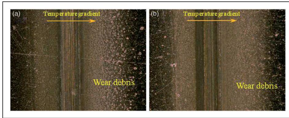
**Figure 6.** The images of wear debris distribution. (a) at temperature gradient of  $3.67^{\circ}\text{C}/\text{mm}$ ; (b) at temperature gradient of  $3.0^{\circ}\text{C}/\text{mm}$ .
