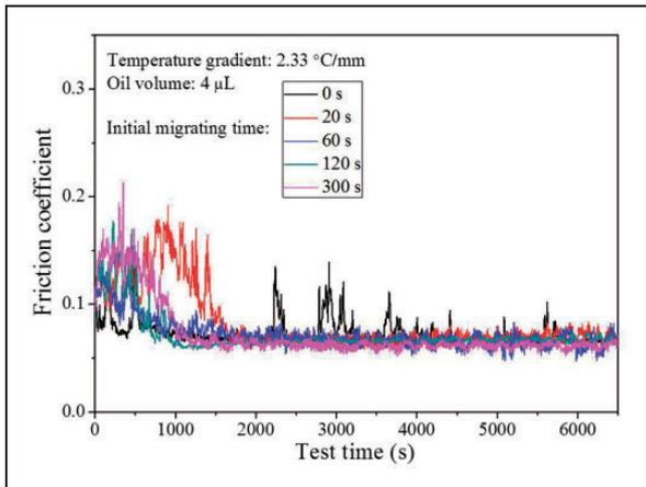
**Figure 9.** Evolution of friction curves under different initial migrating times at temperature gradient of  $2.33^{\circ}\text{C}/\text{mm}$ .
