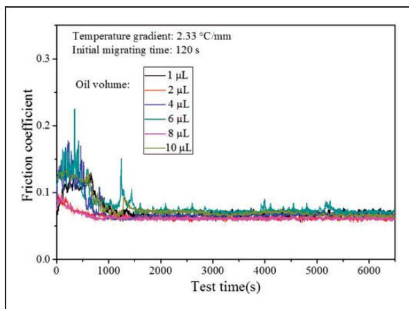
**Figure 7.** Evolution of friction curves under different oil volumes at temperature gradient of  $2.33^{\circ}\text{C}/\text{mm}$ .
