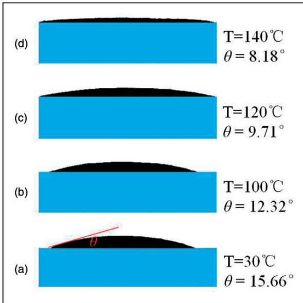
**Figure 3.** Equilibrium contact angle of oil at different temperatures.
