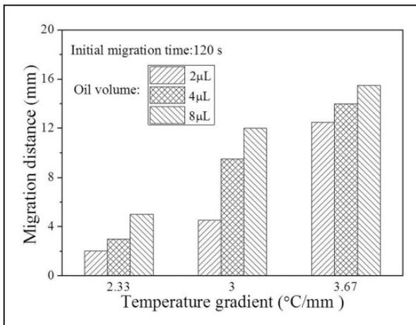
**Figure 4.** The relation between the temperature gradient and migration distance.
