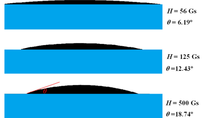
Fig. 4. Equilibrium contact angle of FF under different surface magnetic field intensities.
