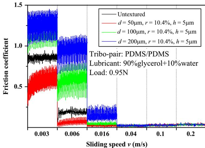
**Fig. 5.** Friction coefficients of untextured and textured PDMS (hydrophobic) with different dimple diameters as a function of sliding speed.
