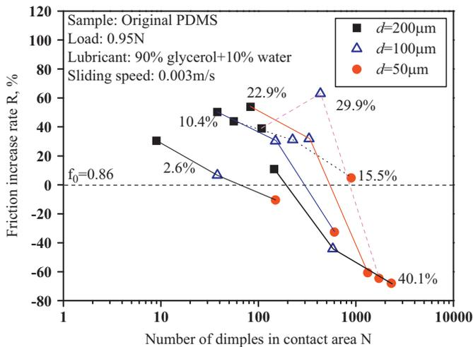
Fig. 8. Surface texture effect on the friction of a hydrophobic PDMS disk sliding against a hydrophobic PDMS pin.
