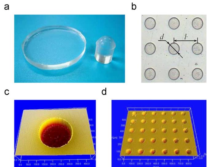
Fig. 2. (a) Image of the tribopair, (b) optical microscope image of a dimple pattern, (c) 3D profile of a dimple and (d) 3D profile of a pattern.
