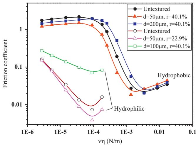
Fig. 7. Stribeck curves of untextured and textured PDMS with different surface wettabilities.
