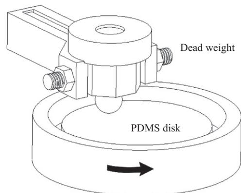
Fig. 4. Schematic diagram of the test setup.
