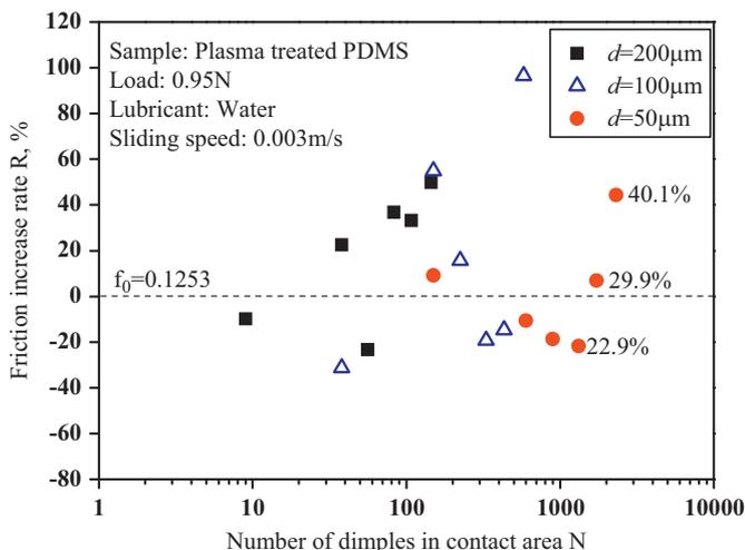
Fig. 9. Surface texture effect on the friction of a hydrophilic PDMS disk sliding against a hydrophobic PDMS pin.
