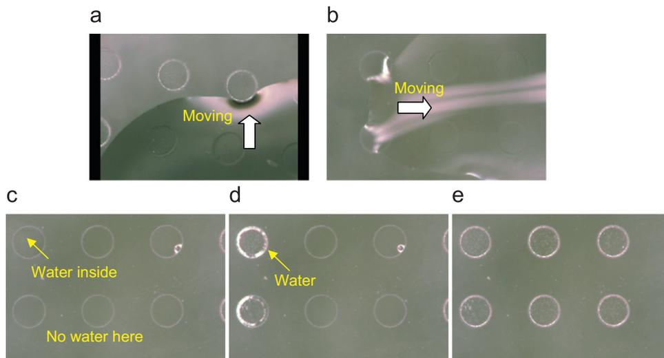
Fig. 10. Behavior of a water drop moving over a textured hydrophobic surface of PDMS.
