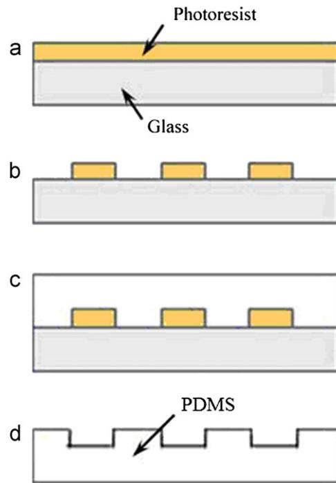
Fig. 1. Procedure of disk preparation and surface texturing for PDMS.
