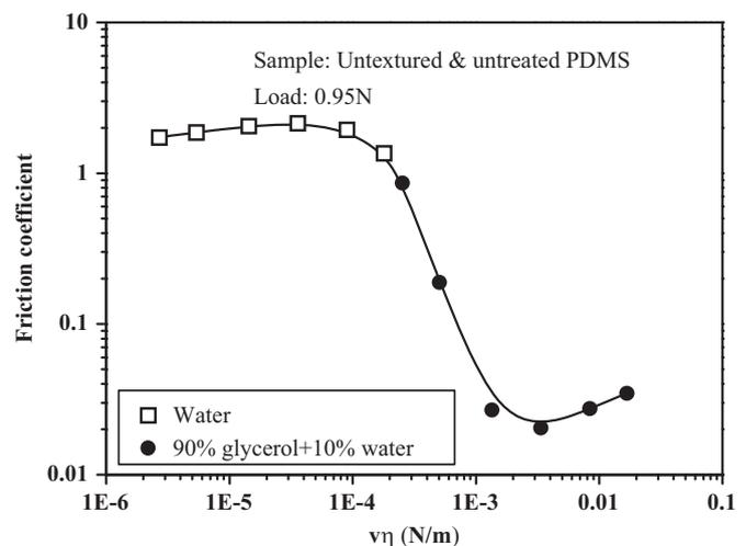
**Fig. 6.** Stribeck curve of untextured and hydrophobic PDMS with water and glycerol solution lubrication.
