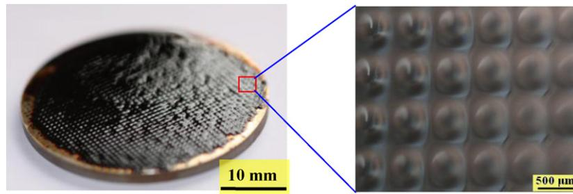
Fig. 3. Photos of magnetic film arrays covered with ferrofluids.
