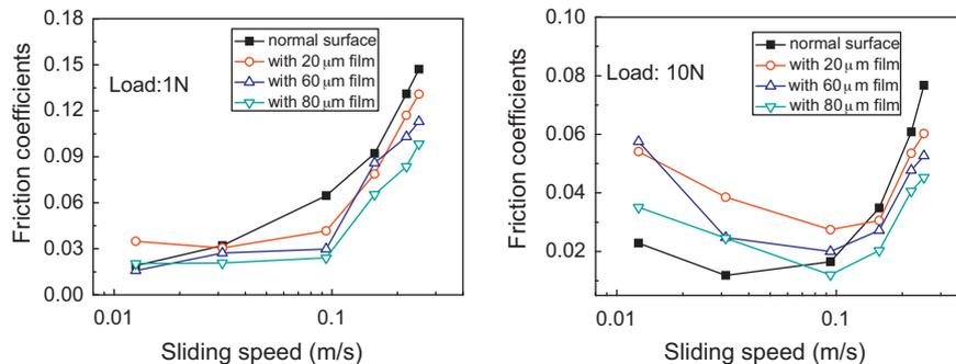
**Fig. 7.** Friction coefficients versus sliding speed of normal surface specimen and specimens with magnetic surface.
