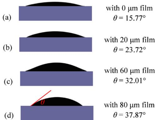
**Fig. 6.** The droplet shapes of FF on normal and magnet arrayed surface.
