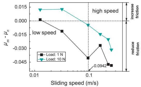
**Fig. 8.** Difference value between  $\mu_m$  (friction coefficient of specimen with 80  $\mu\text{m}$  films) and  $\mu_n$  (friction coefficient of normal surface) when both lubricated with FF.
