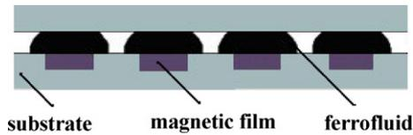
Fig. 1. Design diagram of FF lubrication with magnetic film arrayed surface.
