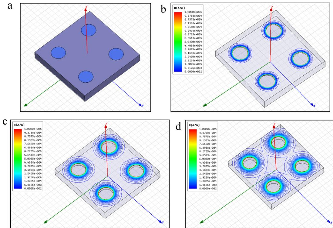
Fig. 4. The calculated magnetic flux density distribution of the arrayed surfaces. (a) Calculation model of the arrayed surface; (b) with 20  $\mu\text{m}$  thickness film; (c) with 60  $\mu\text{m}$  thickness film; (d) with 80  $\mu\text{m}$  thickness film.
