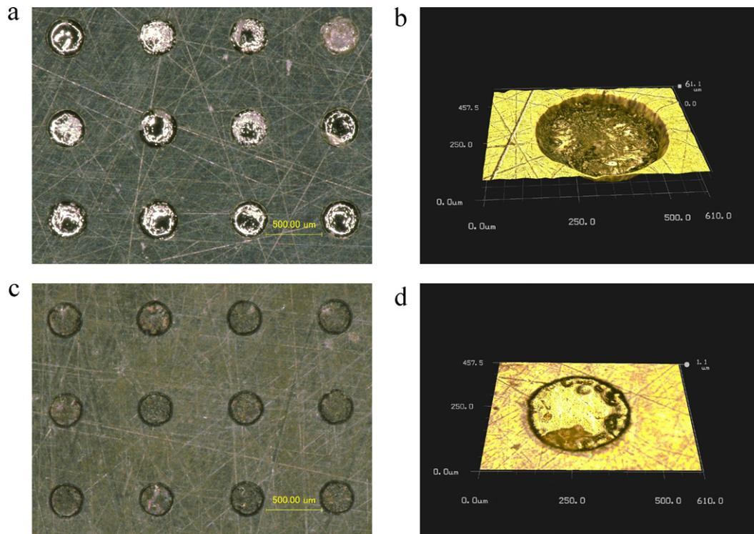
Fig. 2. Surface machining process (a) micro-dimple pattern after electrolytic machining; (b) 3D image of a single micro-dimple; (c) specimen surface after electrodeposition CoNiMnP magnet film; (d) 3D image of a single micro-magnet.
