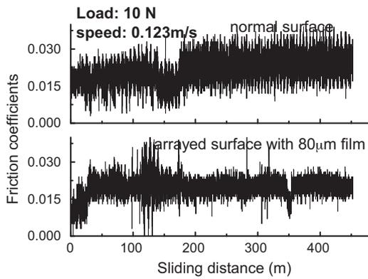
Fig. 9. Variation of friction coefficients during the wear tests.
