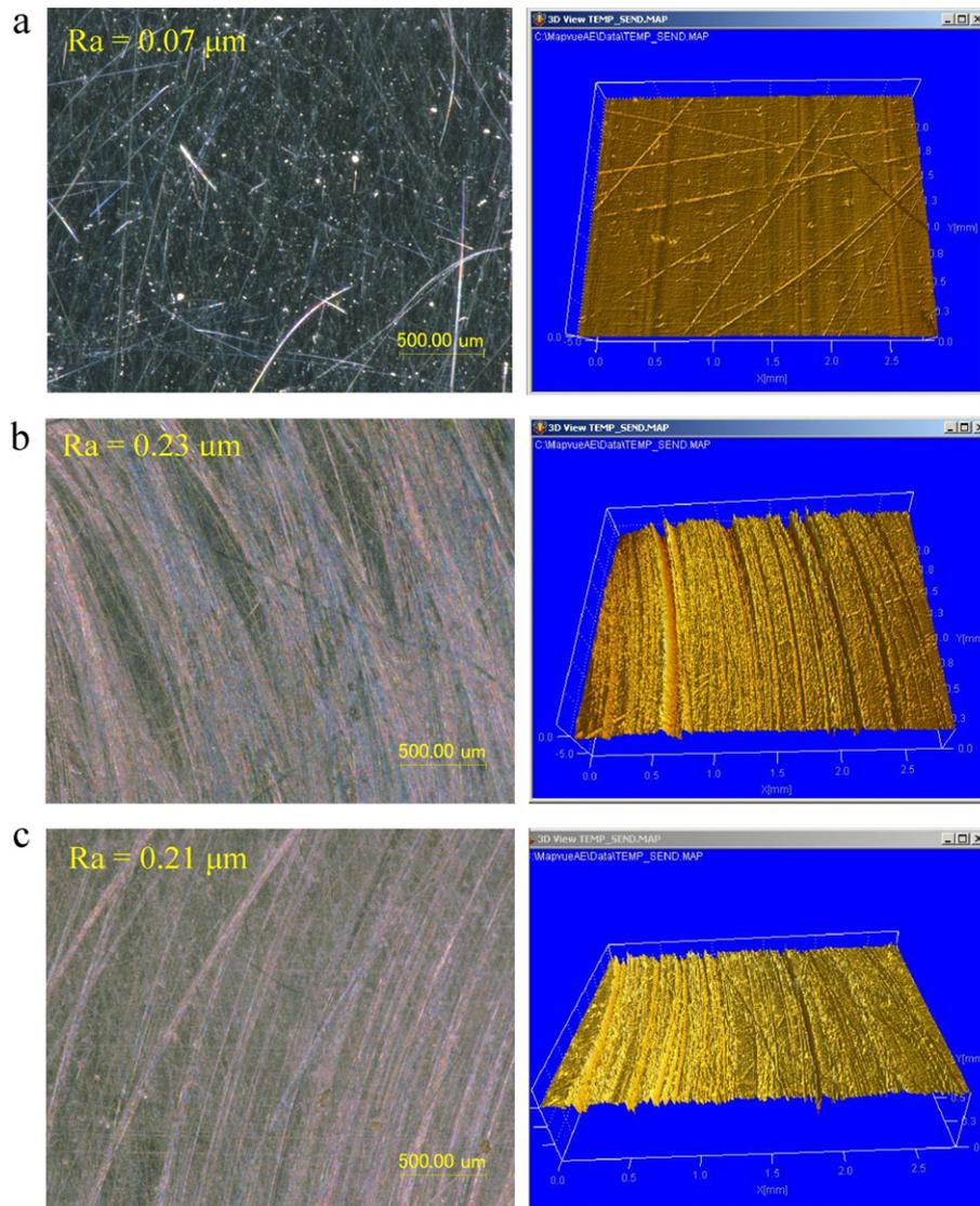
Fig. 10. Optical microscope images and 3D profiles of the upper disks' surfaces (a) before test; (b) opposite specimen with normal surface; (c) opposite specimen with 80  $\mu\text{m}$  magnetic films.
