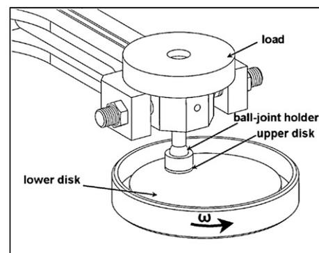
Fig. 5. Schematic diagram of pin-on-disk test rig.
