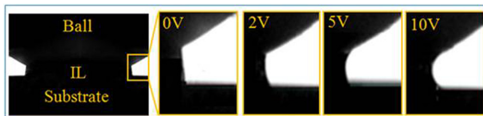
Figure 1. The border image of the IL ([C 2 MIM][BF 4 ]) between the ball and substrate under different EFs.
